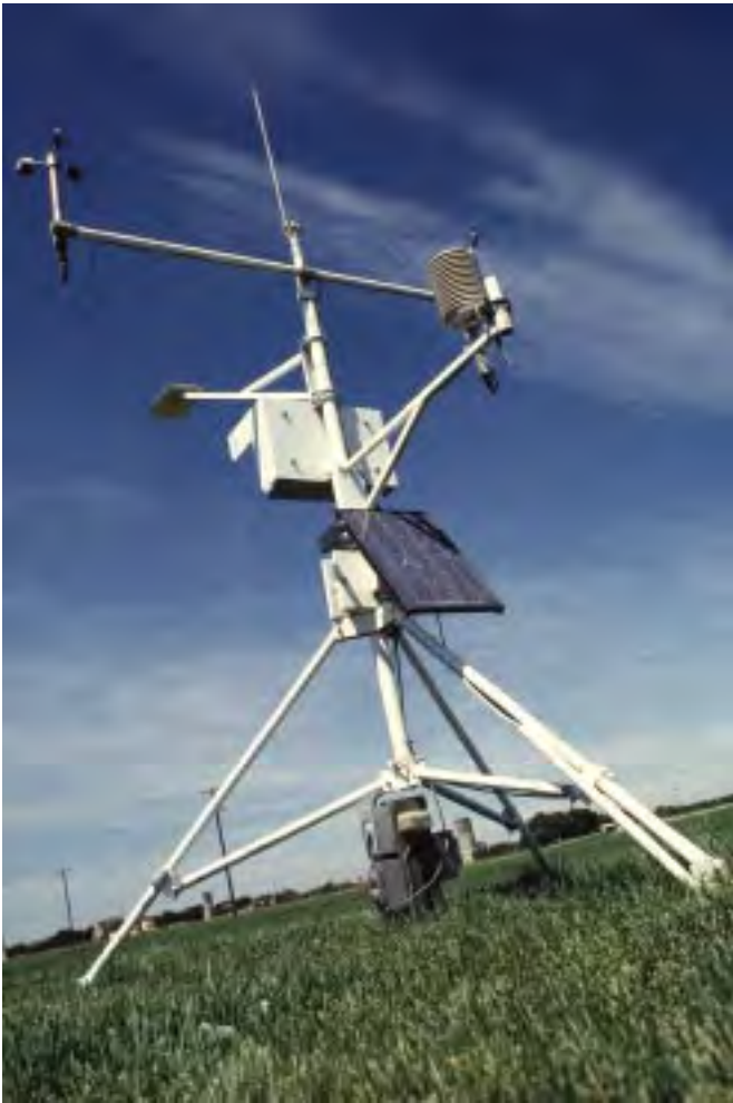
A specialized weather station (CIMIS station) or a Class A evaporation pan (background) can be used to determine reference evapotranspiration (ET c ) for a site. Daily CIMIS data is available online at www.cimis.water.ca.gov .
