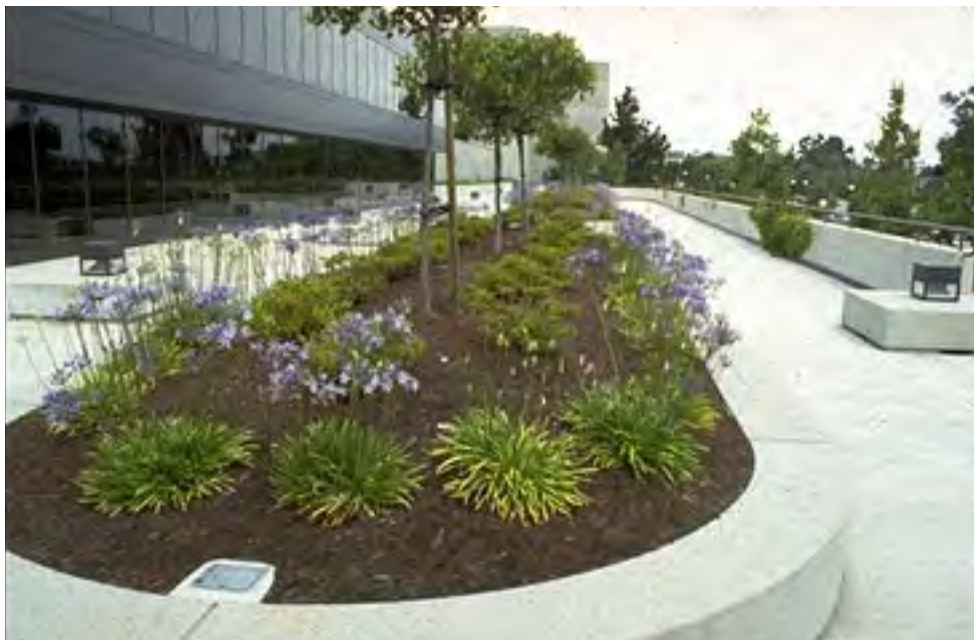
Plantings surrounded by heat-absorbing surfaces, reflective surfaces, or exposed to particularly windy conditions would be assigned a high microclimate value (1.1 - 1.4).
