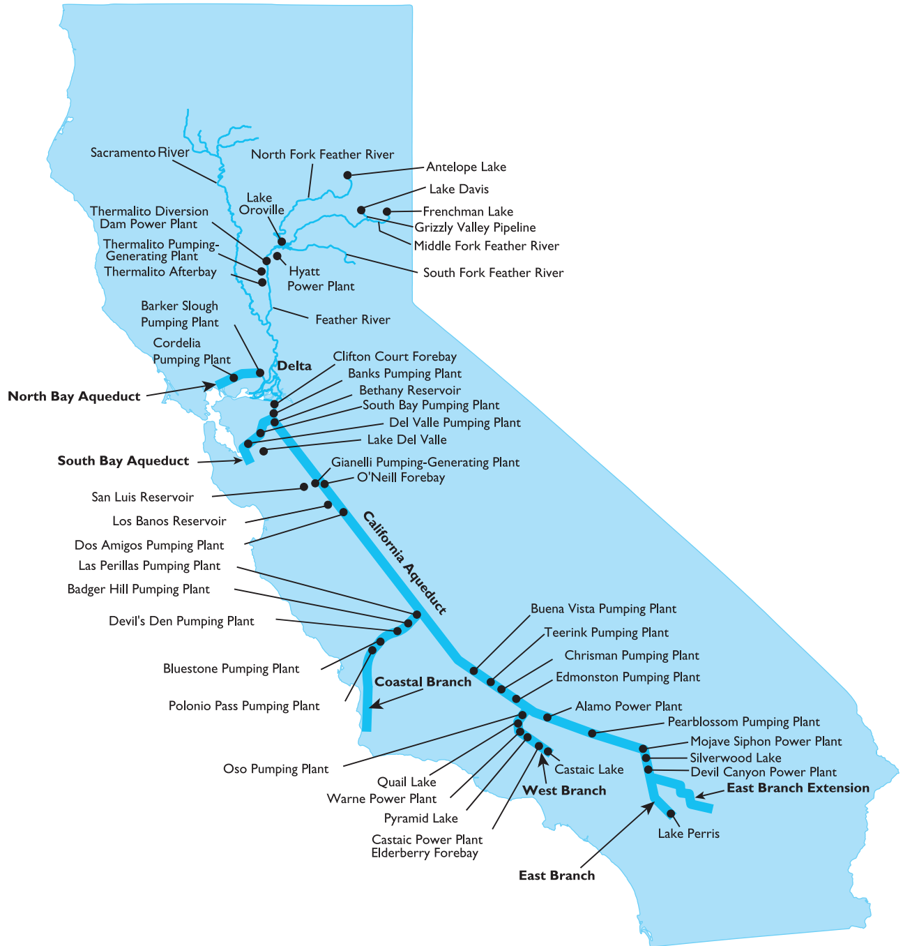
Names and Locations of Primary Water Delivery Facilities
