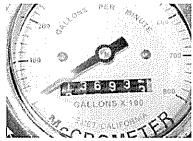
Flowmeter readings are in hundreds of gallons so we must multiply the difference by 100 to get gallons.
