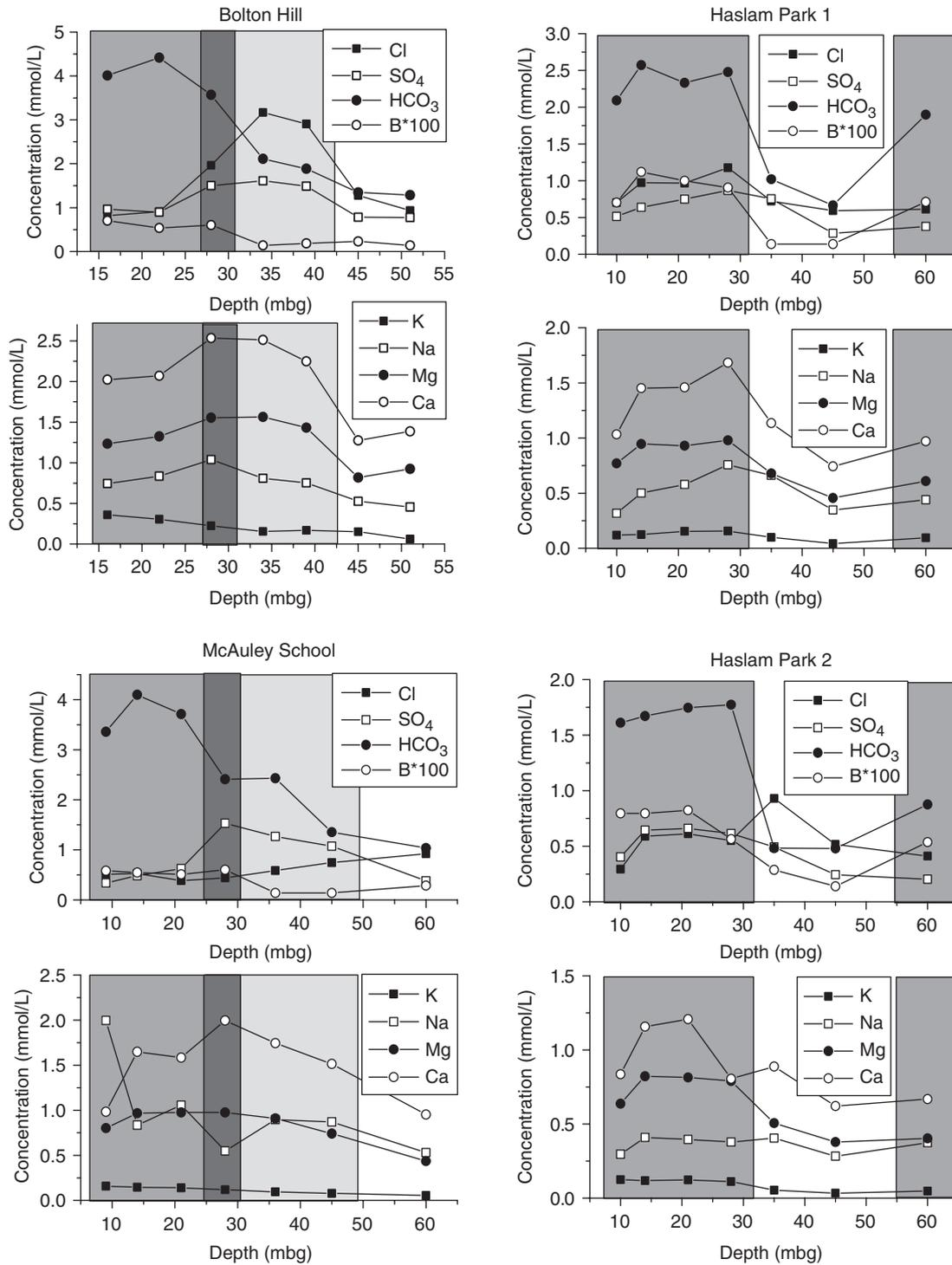
Fig. 5. Mean concentrations plotted against depth below ground. Different chemical signatures are highlighted with shaded areas –dark grey areas showing an admixture of sewage and light grey areas show an alternative source admixture (e.g. stormwater).
