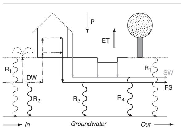
**Fig. 3.** Schematic of the urban water cycle. Dotted lines indicate mains water supply, full lines indicate foul water (black) and stormwater (grey) system.
