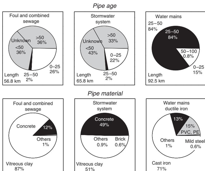
**Fig. 4.** The top row shows age distributions (in years) of the pipe network in Bessacarr with the total length displayed in the bottom left corner. The lower row displays the percentage distribution of pipe materials in use.
