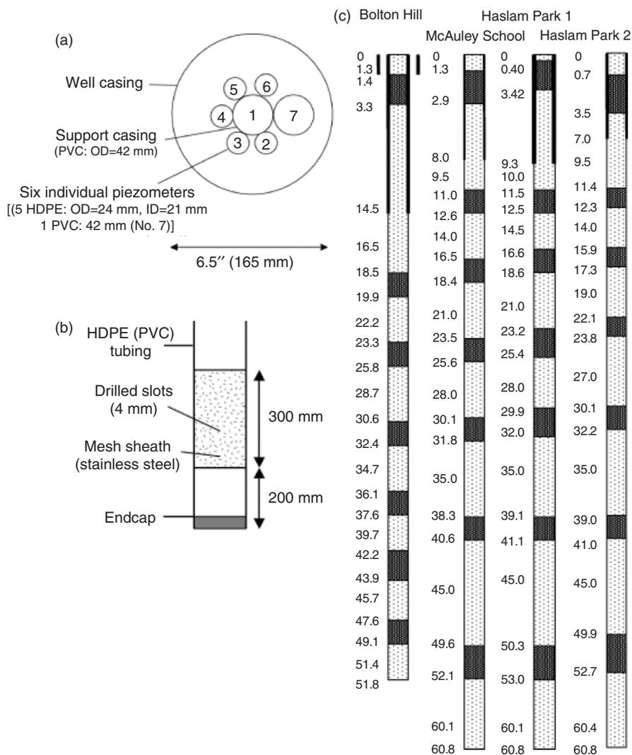
**Fig. 2.** (a) Arrangement of plastic pipes inside the open borehole before backfilling. (b) Detail of screen section showing lowest part of a HDPE (or PVC) pipe with intake section comprising holes drilled into the pipe and covered with a stainless-steel mesh to prevent sand from entering the pipe during sampling. (c) Depths (in metres below ground level) of the seal locations and sampling intervals of each of the four multilevels.
