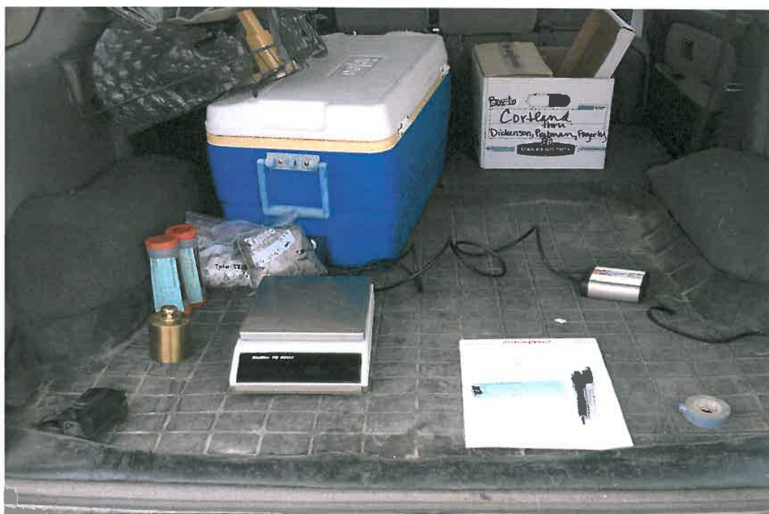
Sample Weighing, Logging and Preparation; upper photo using triple beam balance, lower photo, using electronic scale.
